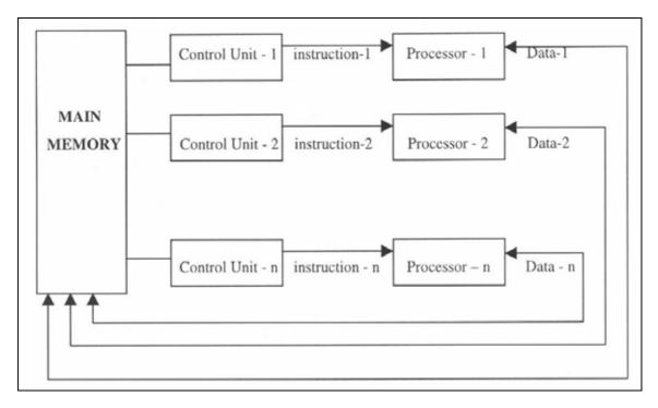
Figure 1. A parallel processor system
