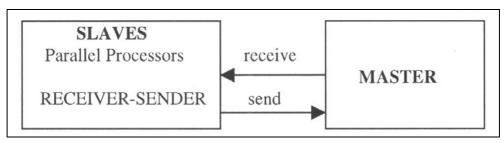
Figure 2. General view of a master-slave for PVM system
