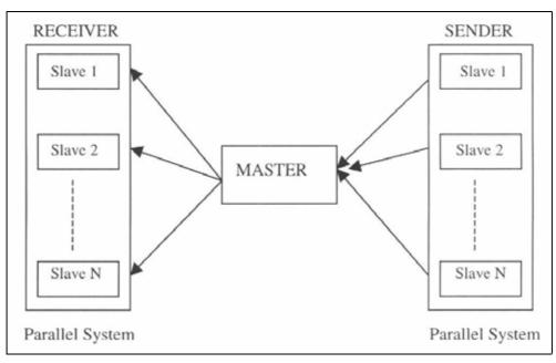
Figure 3. Working principle of a PVM system
