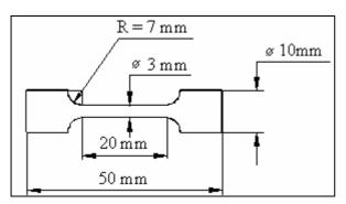
Figure 2. Schematic representation of tensile specimen
