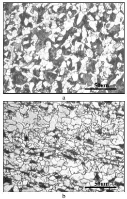
Figure 3. Microstructure of medium carbon (a) and low carbon (b)
