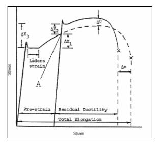
$\Delta Y1$  = Increase in stress produced by pre-strain;  $\Delta Y2$  = Increase in stress produced by ageing;  $\Delta Y3$  = Increase in stress due to prestraining and ageing =  $\Delta Y1 + \Delta Y2$ ;  $\Delta U$  = Change in UTS due to pre-straining and ageing;  $\Delta e$  = Change in total elongation due to pre-straining and ageing
