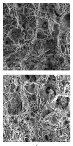
Figure 5. Fracture surfaces of steel 1(a) and steel 2 (b) pre-strained 5 % and than aged at 300  $^{\circ}\!C$  for 1 hour
