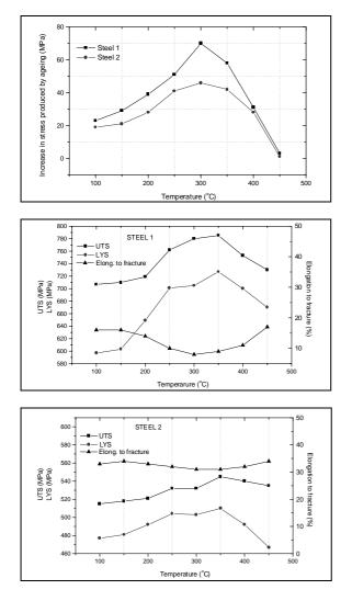
Figure 4. The effect of the static strain ageing on mechanical properties of microalloyed steels prestrained 5% and than aged at different temperatures
