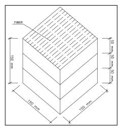
Figure 1. Shape of samples of mud bricks (A1-B1-C1-D1)
