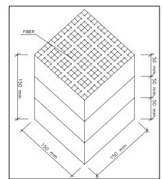
Figure 2. Shape of samples of mud bricks (A2-B2-C2-D2)
