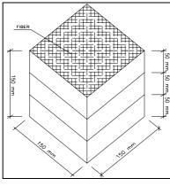
Figure 3. Shape of Samples of Mud Bricks (A3-B3-C3-D3)
