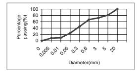
Figure 4. Grading curve from particle size analysis of clay-basaltic pumice-cement used for the preparation of specimens (ASTM and Turkish Standard requirement) (TS 2514, 2515).
