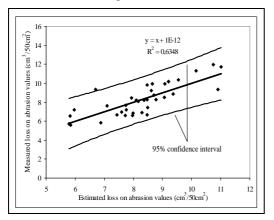
Figure 4. Comparison of experimental and calculated loss on abrasion values
