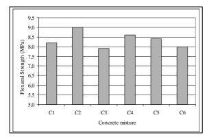
Figure 2. 28 day flexural strength test results
