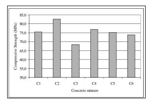
Figure 1. 28 day compressive strength test results.
