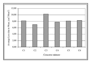
Figure 3. 28 day loss on abrasion test results
