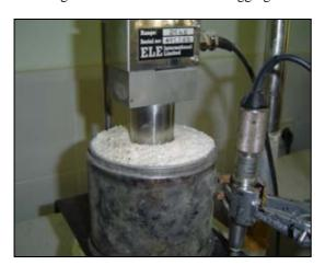
Figure 2. CAR test apparatus.
