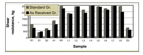
Figure 4. CAR test results of fine aggregates.
