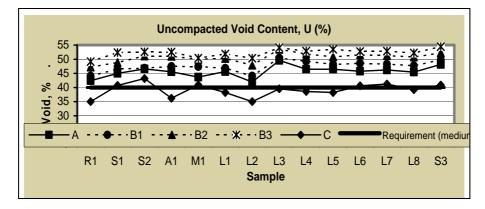
Figure 3. Uncompacted void content of fine aggregates (ASTM C 1252).
