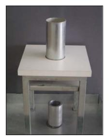
Figure 1. Uncompacted void content apparatus.
