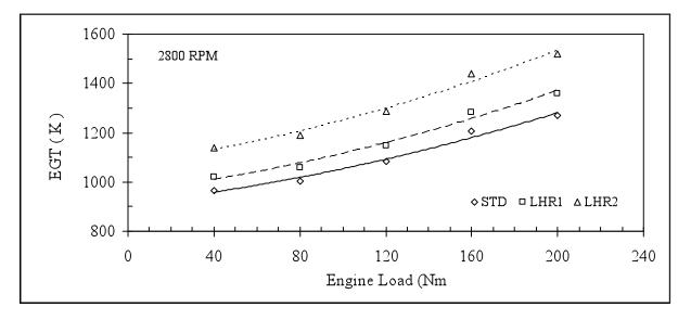
Figure 5. Comparison of EGT by engine load at 2800 rpm.
