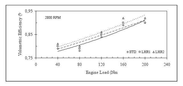
Figure 9. Comparison of volumetric efficiency by engine load at 2800 rpm.
