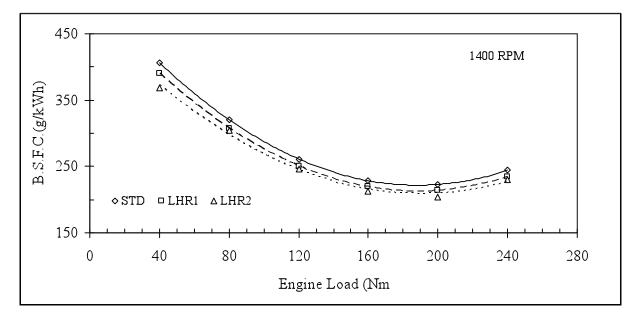
Figure 2. Comparison of BSFC by engine load at 1400 rpm.
