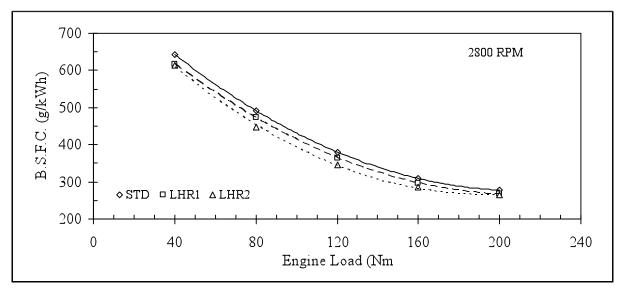
Figure 3. Comparison of BSFC by engine load at 2800 rpm.
