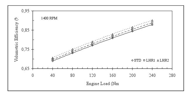
Figure 8. Comparison of volumetric efficiency by engine load at 1400 rpm.
