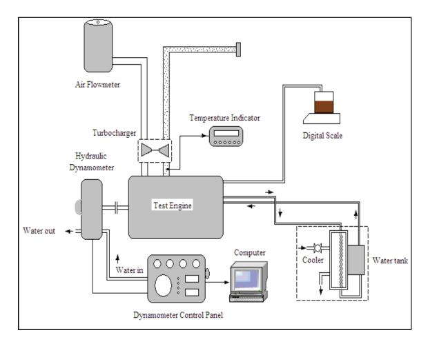
Figure 1. Schematics of test set-up.
