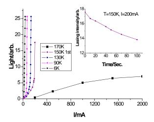
FIG. 1 CURRENT-LIGHT RELATIONSHIPS AT DIFFERENT TEMPERATURES WITH LASER RAPID DEGRADATION AS A FUNCTION OF TIME AT 150K INSET AND NO LASING FOUND AT 170K.
