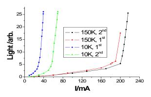
FIG. 2 CURRENT-LIGHT RELATIONSHIPS AT 10K AND 150K, WHERE 1<sup>ST</sup> IS THE INITIAL TEST WITH DEGRADATION HAPPENED AT 150K AND THE 2<sup>ND</sup> IS THE REPEATED TEST AFTER LASING DEGRADATION.
