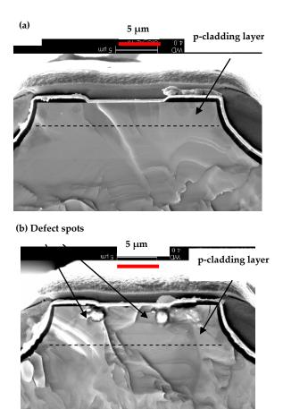
FIG. 5 (a) SEM PROFILE FOR LASER STRUCTURE, WHERE P-CLADDING REGION IS OVER THE DASH LINE. (b) TWO DEFECT SPOTS PRODUCED BY DRIVING CURRENT
