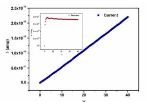
FIG. 10 I-V AND R-V CHARACTERISTICS OF CU25(IN16GA9)SE40TE10 THIN FILM AT ROOM TEMPERATURE
