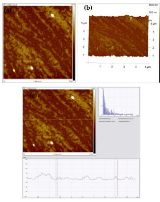
FIG. 7 (A, B, C) AFM SURFACE MORPHOLOGY, THREE DIMENSIONAL VIEW AND ROUGHNESS PARAMETER PROFILE FOR Cu20(IN14GA9)SE45TE12 THIN FILM
