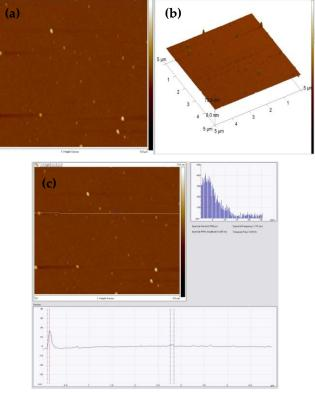
FIG. 8 (A, B, C) AFM SURFACE MORPHOLOGY, THREE DIMENSIONAL VIEW AND ROUGHNESS PARAMETER PROFILE FOR CU25(IN16GA9)SE40TE10 THIN FILM
