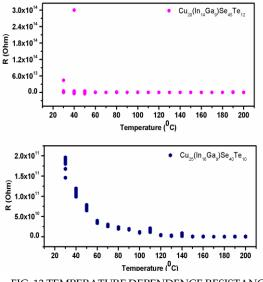
FIG. 13 TEMPERATURE DEPENDENCE RESISTANCE VARIATIONS OF CU25(IN16GA9)SE40TE10 AND CU20(IN14GA9)SE45TE12 THIN FILMS UNDER UNDER APPLIED VOLTAGE RANGE UPTO 40V
