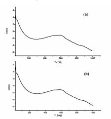
FIG. 4 (A, B) DIFFERENTIAL THERMAL ANALYZER SIGNALS FOR Cu20(IN14GA9)SE45TE12 ALLOY
