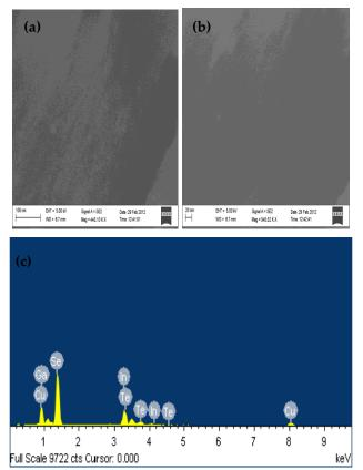
FIG. 2 (A, B, C) FIELD EMISSION SCANNING MICROSCOPE SURFACE MORPHOLOGY AND EDS RESULT FOR CU20(IN14GA9)SE45TE12 ALLOY
