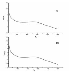
FIG. 5 (A, B) DIFFERENTIAL THERMAL ANALYZER SIGNALS FOR CU25(IN16GA9)SE40TE10 ALLOY
