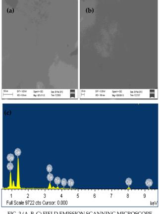
FIG. 3 (A, B, C) FIELD EMISSION SCANNING MICROSCOPE SURFACE MORPHOLOGY AND EDS RESULT FOR CU25(IN16GA9)SE40TE10 ALLOY
