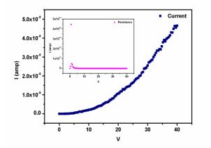
FIG. 9 I-V AND R-V CHARACTERISTICS FOR CU20(IN14GA9)SE45TE12 THIN FILM AT ROOM TEMPERATURE
