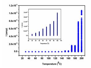
FIG. 12 TEMPERATURE DEPENDENCE CURRENT VARIATION OF Cu25(In16Ga9)Se40Te10 THIN FILM UNDER APPLIED VOLTAGE RANGE UPTO 40V
