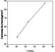
Figure 6. Variation of hardness with load for BTSN-Kcl crystal
