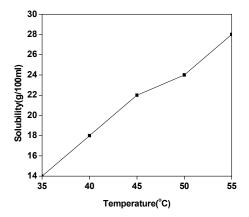
Figure 2. Solubility curve of BTSN-Kcl crystals
