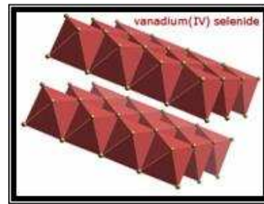
(b) Crystal structure of \text{VSe}_2 single crystal.
