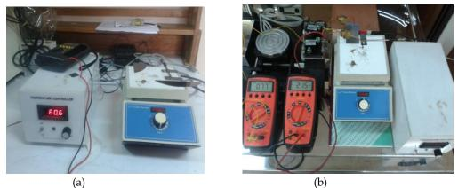
**Image 1**. (a) Conventional hot plate with temperature controller (b) Hot probe measurement experimental set up.
