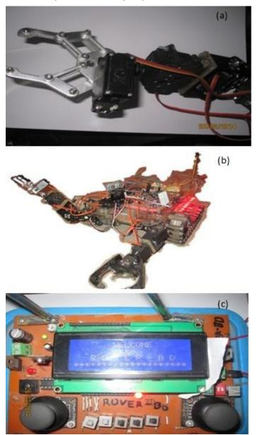
**Figure 1** Construction of the proposed robot. (a) Mechanical arm (b) full body of the robot and | (c) Control and Display unit.
