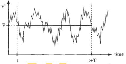
Figure 1. Reynolds averaging illustration of turbulent velocity (v, v')
