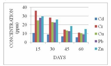
Figure 2 Reduction of Cd, Cr, Cu, Pb and Zn in Pot No. B1 to B4
