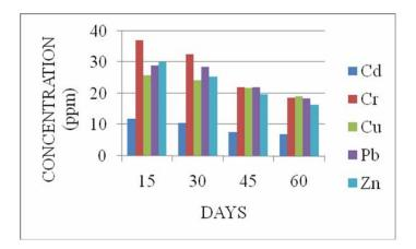
Figure 5 Reduction of Cd, Cr, Cu, Pb and Zn in Pot No. E1 to E4
