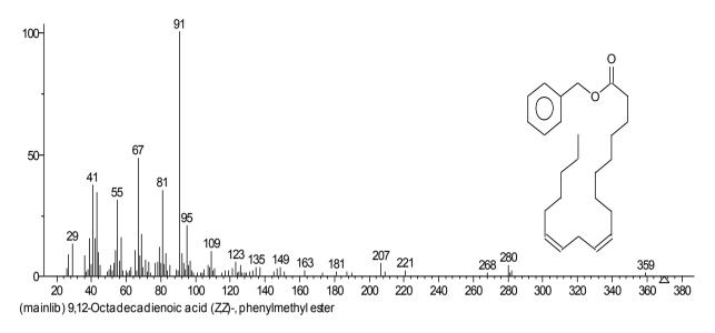
Fig 2: Mass spectrum of 9,12-Octadecadienoic acid (Z,Z)-, phenylmethyl ester
