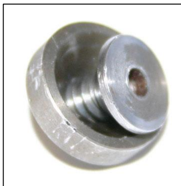
Figure 1 Proprietary Screw on Google Mini Search Appliance (Clark, 2005)
