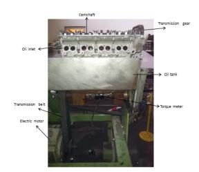
Figure 3. Camshaft wear test machine
