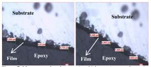
Figure 7. Manganese phosphate coating thickness a)cam peak, coating thickness between 6,7 to 8  $\mu m$  b) cam flank area, coating thickness between 6,8 to 8,5  $\mu m$
