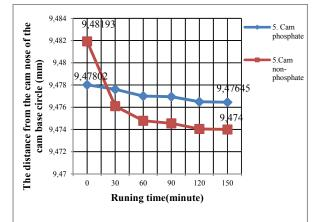
Figure 11. The change on the points of the 5th cam on phosphated and non-phosphated camshafts
