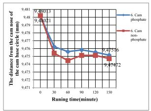
Figure 12. The change on the points of the 6th cam on phosphated and non-phosphated camshafts
