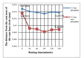
Figure 9. The change on the points of the 3rd cam on phosphated and non-phosphated camshafts
