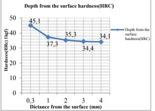
Figure 5. Material hardness depth of the surface
