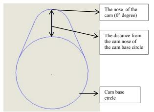
Figure 8. The cut view of the cams on the camshafts and the parts on the cam.
