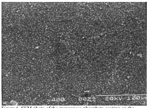
Figure 6. SEM photo of the manganese phosphate coating on the chilled ductile iron camshaft
