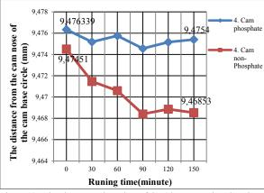
Figure 10. The change on the points of the 4th cam on phosphated and non-phosphated camshafts
