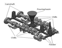
Figure 1. Camshaft model and chills assembly on camshafts
