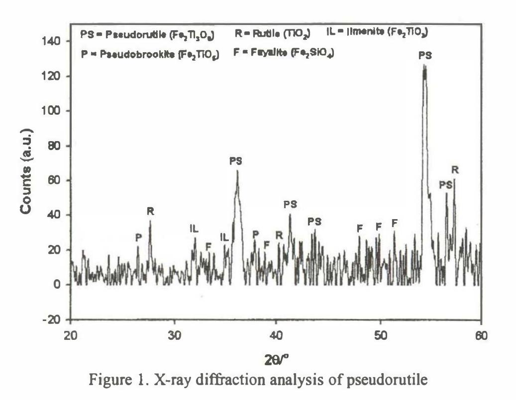
Pseudorutile was obtained from Eczacıbaşı Doğa Madencilik Tic.A.Ş. TiO<sub>2</sub> and Fe<sub>2</sub>O<sub>3</sub> contents in pseudorutile, analyzed by X-ray fluorescence (XRF) analysis, are 50.15% and 22.67%, respectively.
