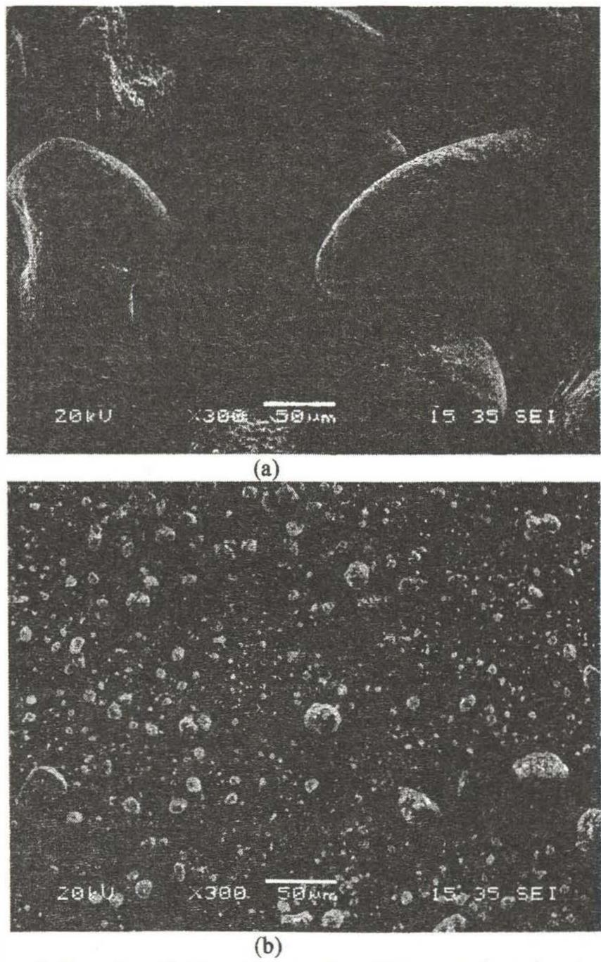
Figure 2. Scanning electron micrographs of (a) non-activated and (b) activated pseudorutile for 30 min.
