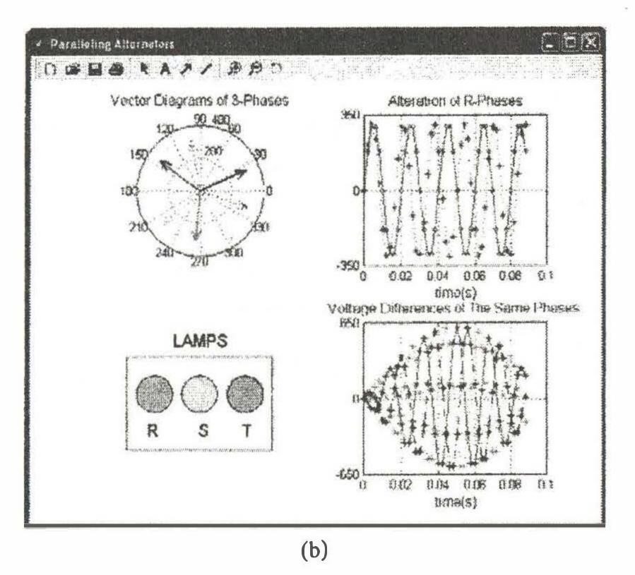
Figure 5. Instantaneous positions of the dynamic animation of paralleling alternators, a) t=0.03s, b) t=0.088s
