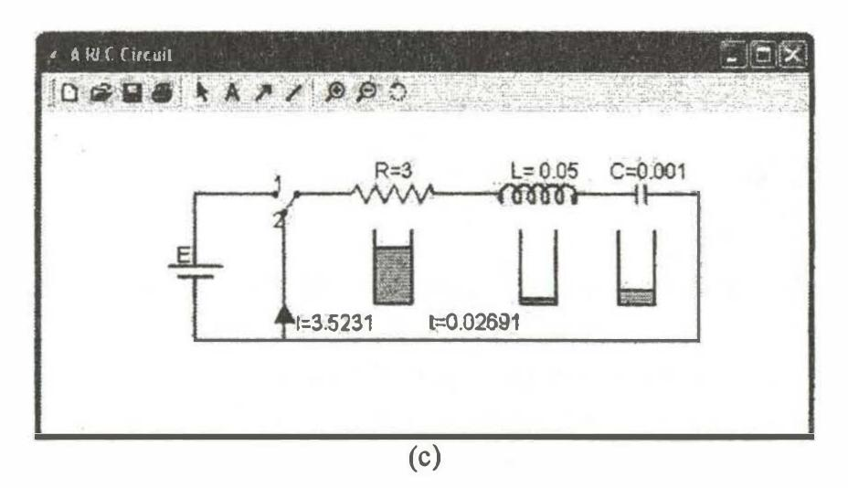
Figure 3.a) Graphical representations of the selected circuit parameters, b,c) Instantaneous schematics of the dynamic animation of the circuitry at the instant t=0.015954s and t=0.02691s.
