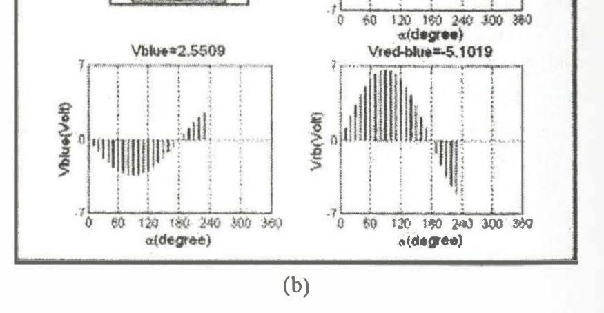
Figure 4. Instantaneous positions of the dynamic animation of the ac voltage generator at the position of, a)  $\alpha = 120^{\circ}$ , b)  $\alpha = 230^{\circ}$ .
