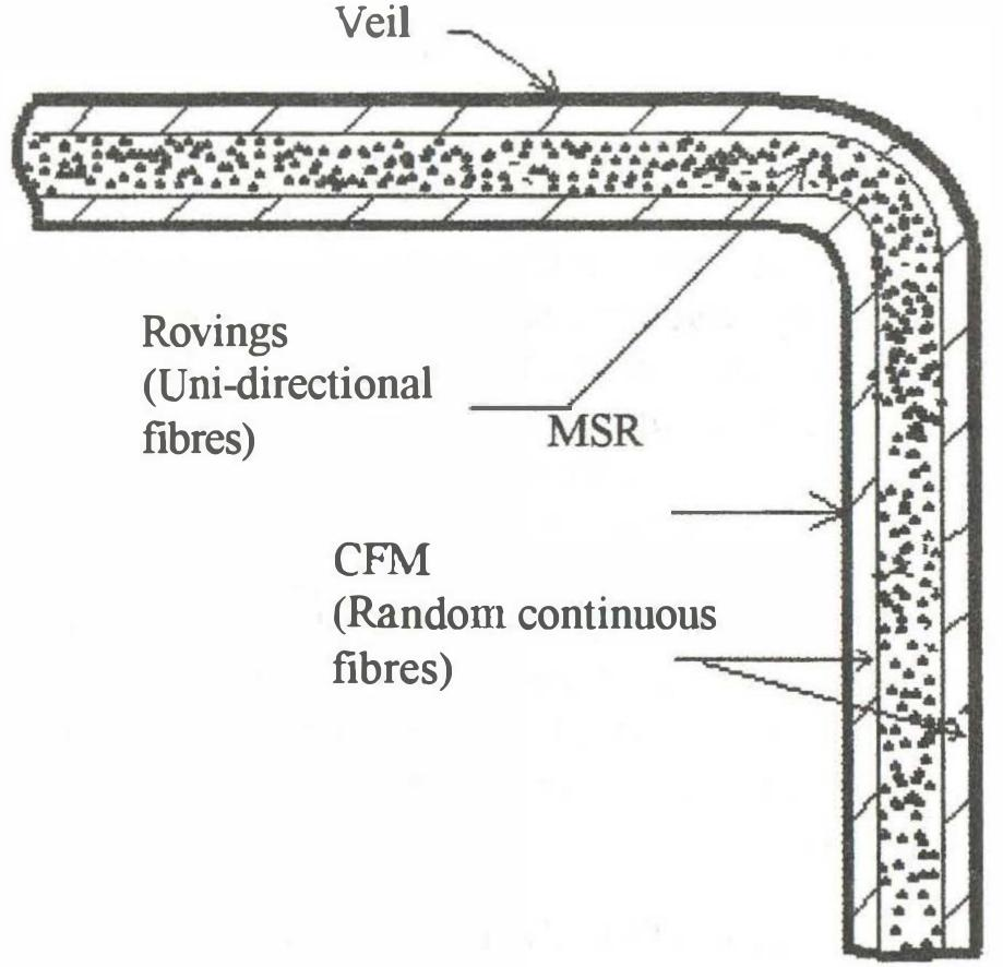
Fig. 1. Typical construction of a pultruded GRP box section.
