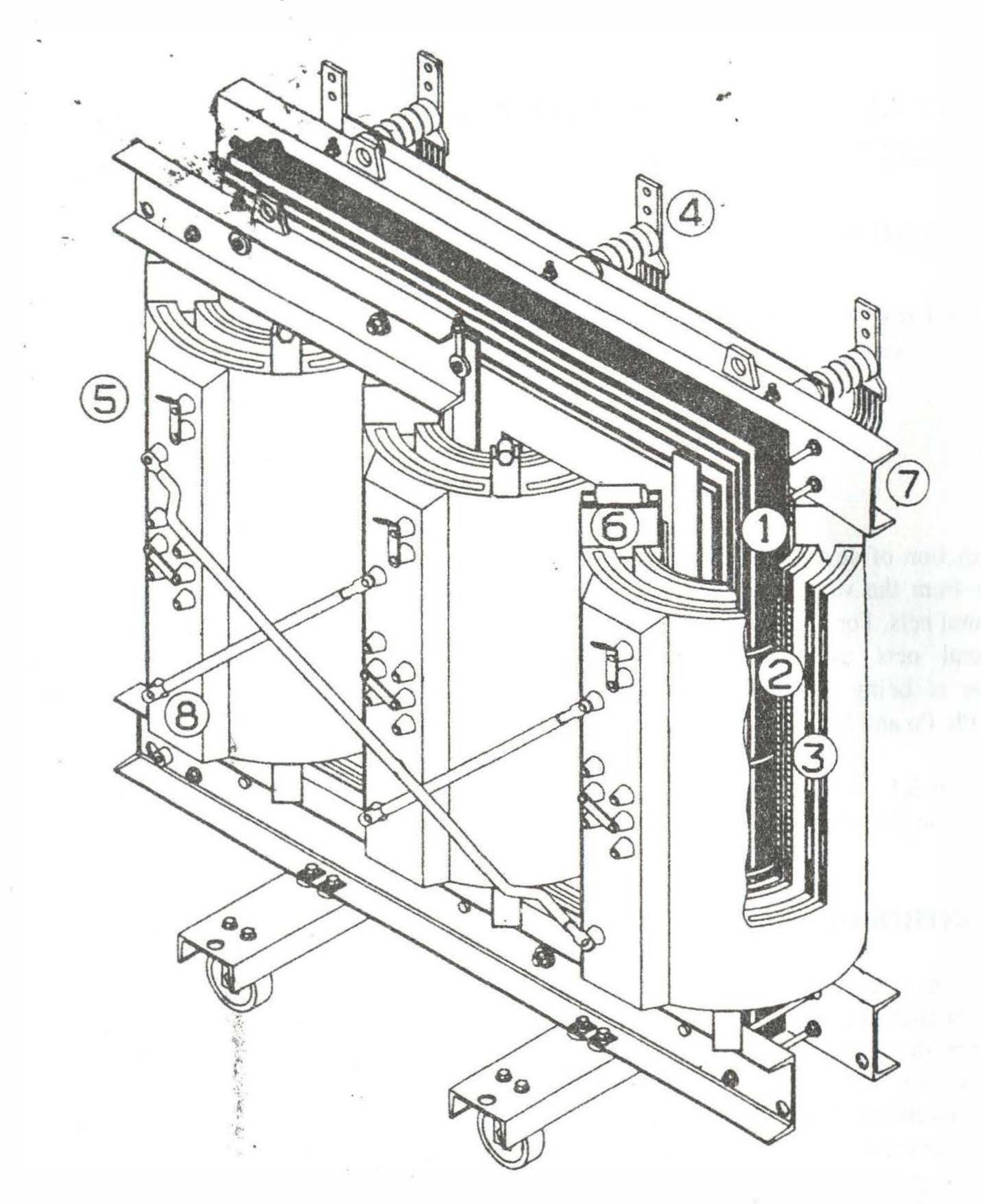
Figure 1. General structure of a GETI cast resin transformer (1-Core, 2.3-Both LV and HV winding, 4-LV terminals, 5-HV terminals and tappings, 6-Resilent spacers, 7-Yoke clamping and wheel frame, 8-Fiberglass reinforced epoxy
