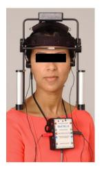
Fig. 4. JT-3D\* Jaw Tracker used together with EMG to monitor a bite registration
