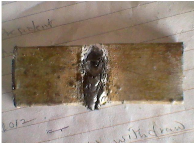
Plate 1: A Welded Sample Work Piece before Machining
