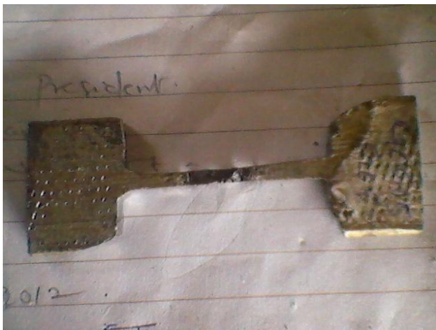
Plate 2: Prepared Sample for Testing After Machining
