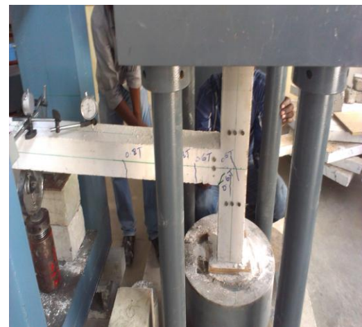
Fig 4 Testing of Beam column joint
