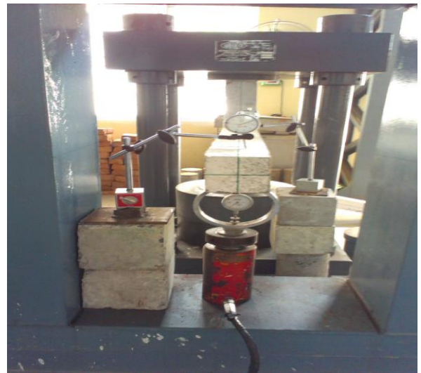
Fig 3 Experimental setup for Beam Column joint
