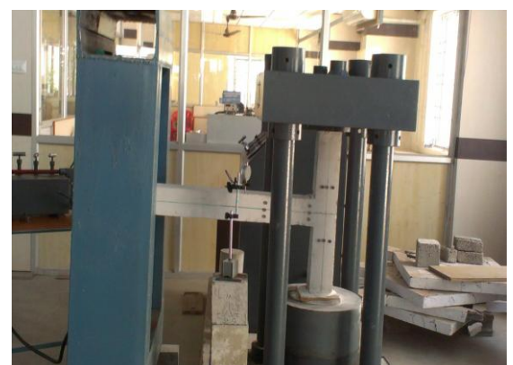
Fig 5 Side view of loading frame with testing specimen
