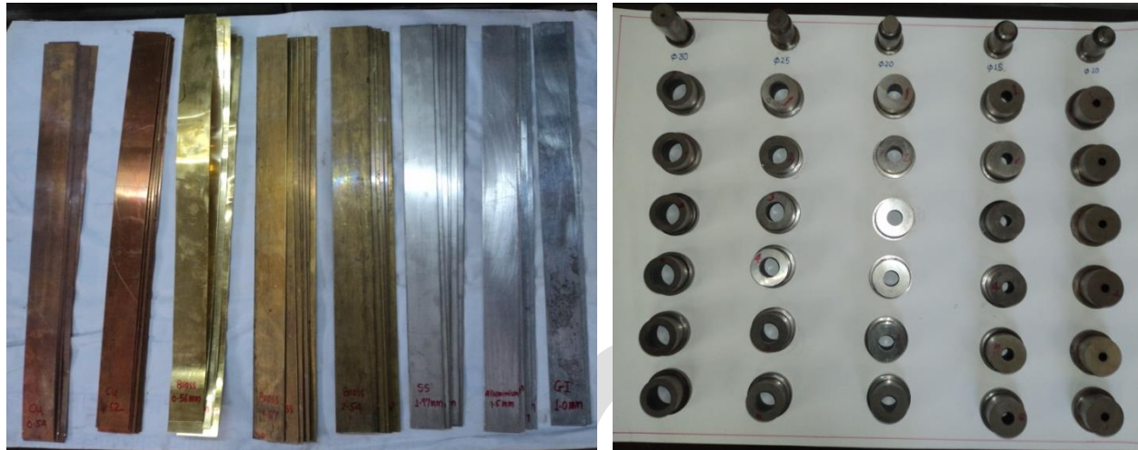
Figure 3. Photograph shows varying thicknesses of sheet metals and punches
