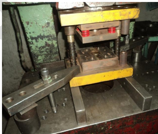
Figure 2. Photograph of the simple die loaded on the used press
