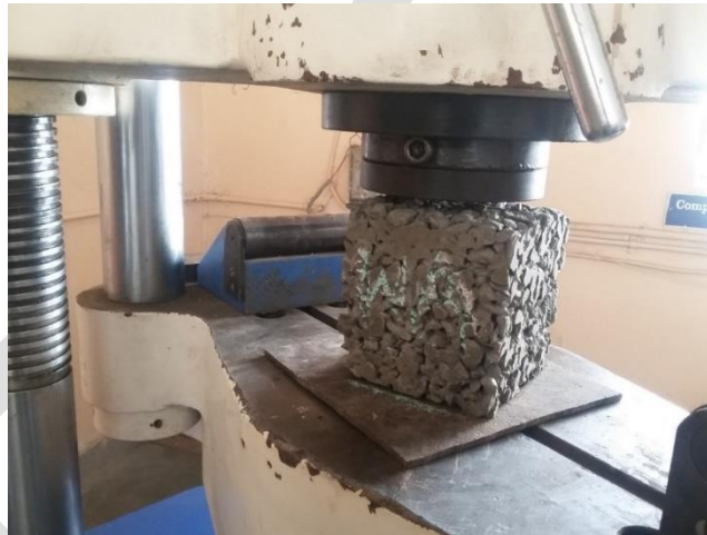
Fig. 5. Compressive strength test
