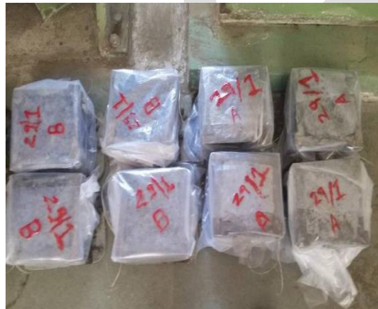
Figure 4. Curing of concrete
