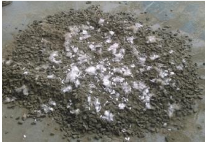
Fig.3. Mixing of polypropylene fiber in concrete
