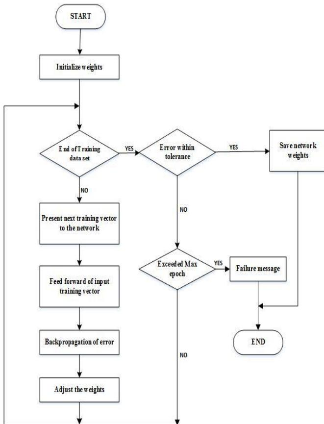
Figure 5: Block Diagram of Back propagation Neural Network.
