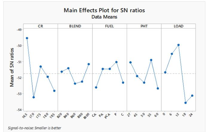
**Fig.4: SN Ratio for NOx**
