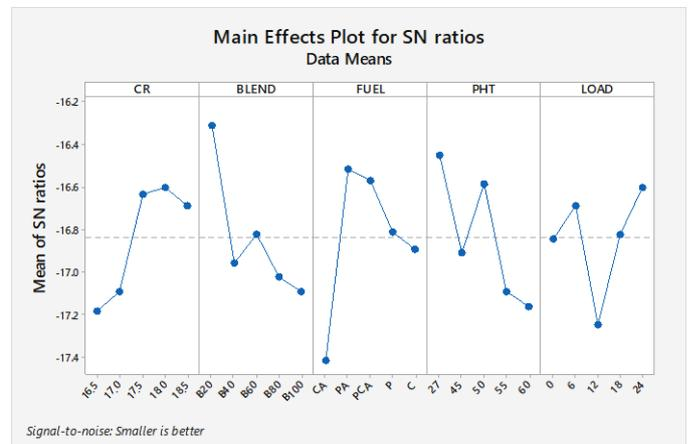
**Fig.6: SN Ratio for Brake Thermal Efficiency**
