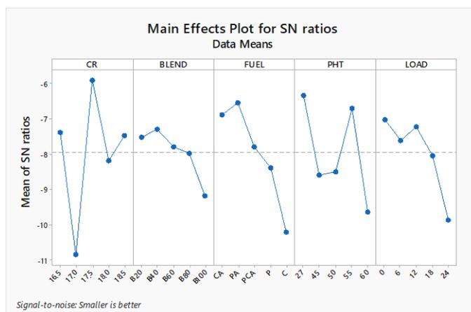
Fig.2: SN Ratio for CO<sub>2</sub>
