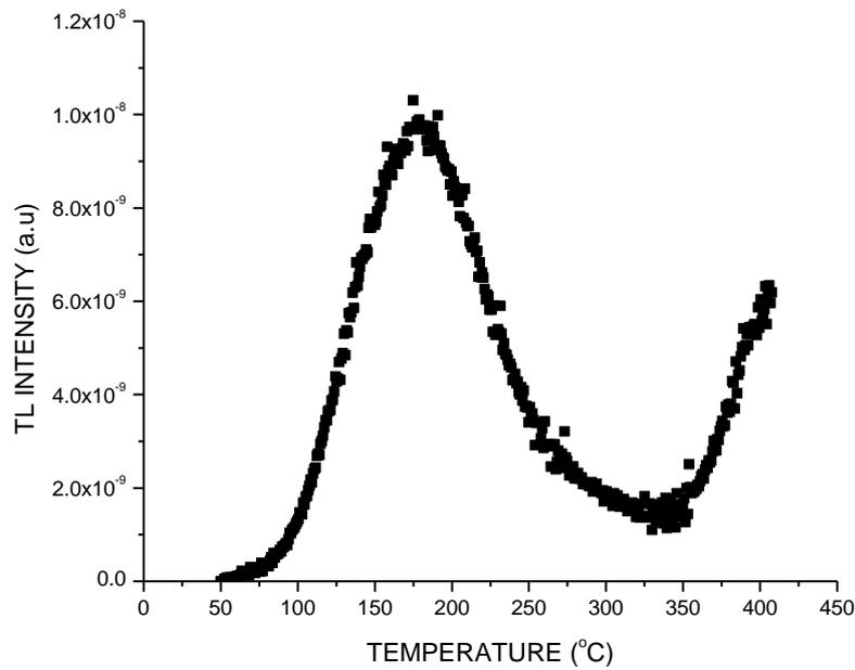
Fig.1: Glow curve of synthetic Fused quartz with 5 °C/s heating rate using <sup>60</sup>Co with irradiation for 1h
