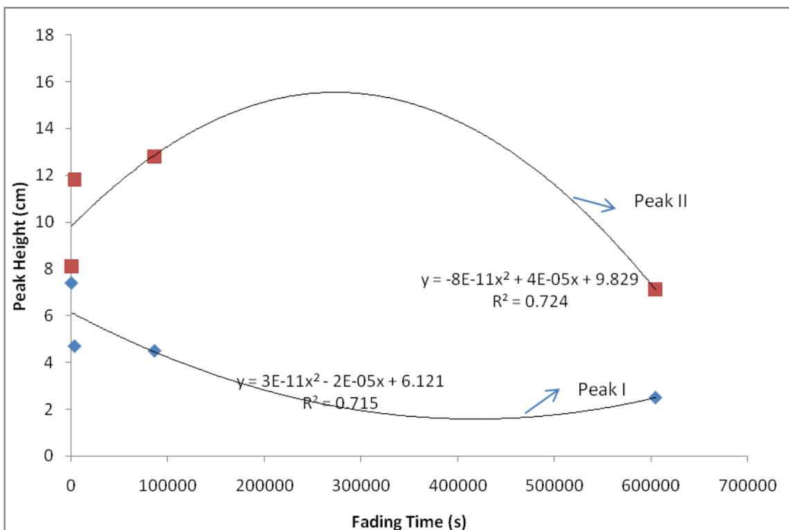
Fig. 6: Fading pattern of synthetic fused quartz with <sup>60</sup>Co irradiation source
