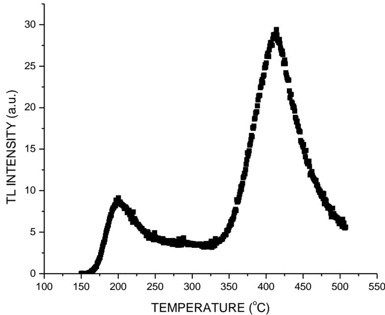
Fig. 3: Glow curve of synthetic Fused quartz with 5 °C/s heating rate and 150 °C preheat using  $^{60}\text{Co}$  source with irradiation for 1 h
