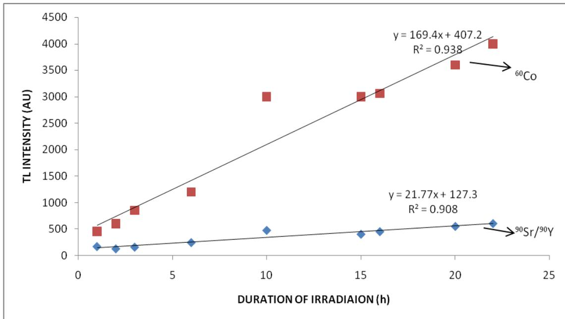
Fig. 5: Dose response of synthetic Fused quartz with <sup>60</sup>Co and <sup>90</sup>Sr/<sup>90</sup>Y irradiation sources respectively
