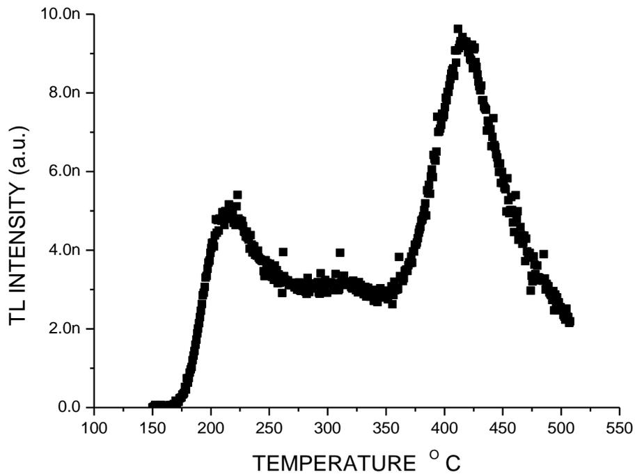
Fig.4: Glow curve of synthetic Fused quartz with 5 °C/s cycle time and 150 °C preheat using  $^{90}\text{Sr}/^{90}\text{Y}$  source with irradiation for 1 h
