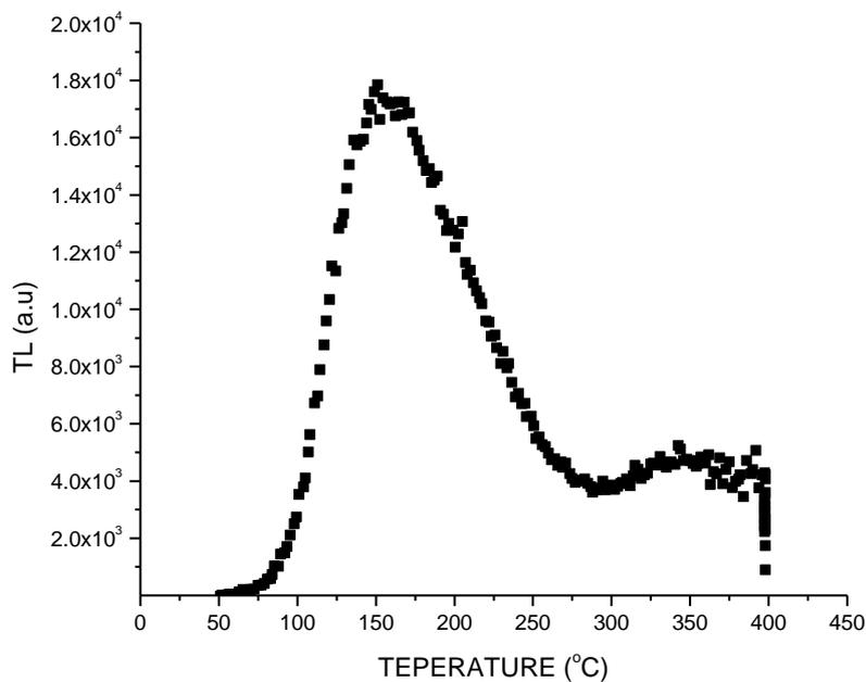
Fig. 2: Glow curve of synthetic Fused quartz with 5 °C/s heating rate using <sup>90</sup>Sr/<sup>90</sup>Y source with irradiation for 1 h
