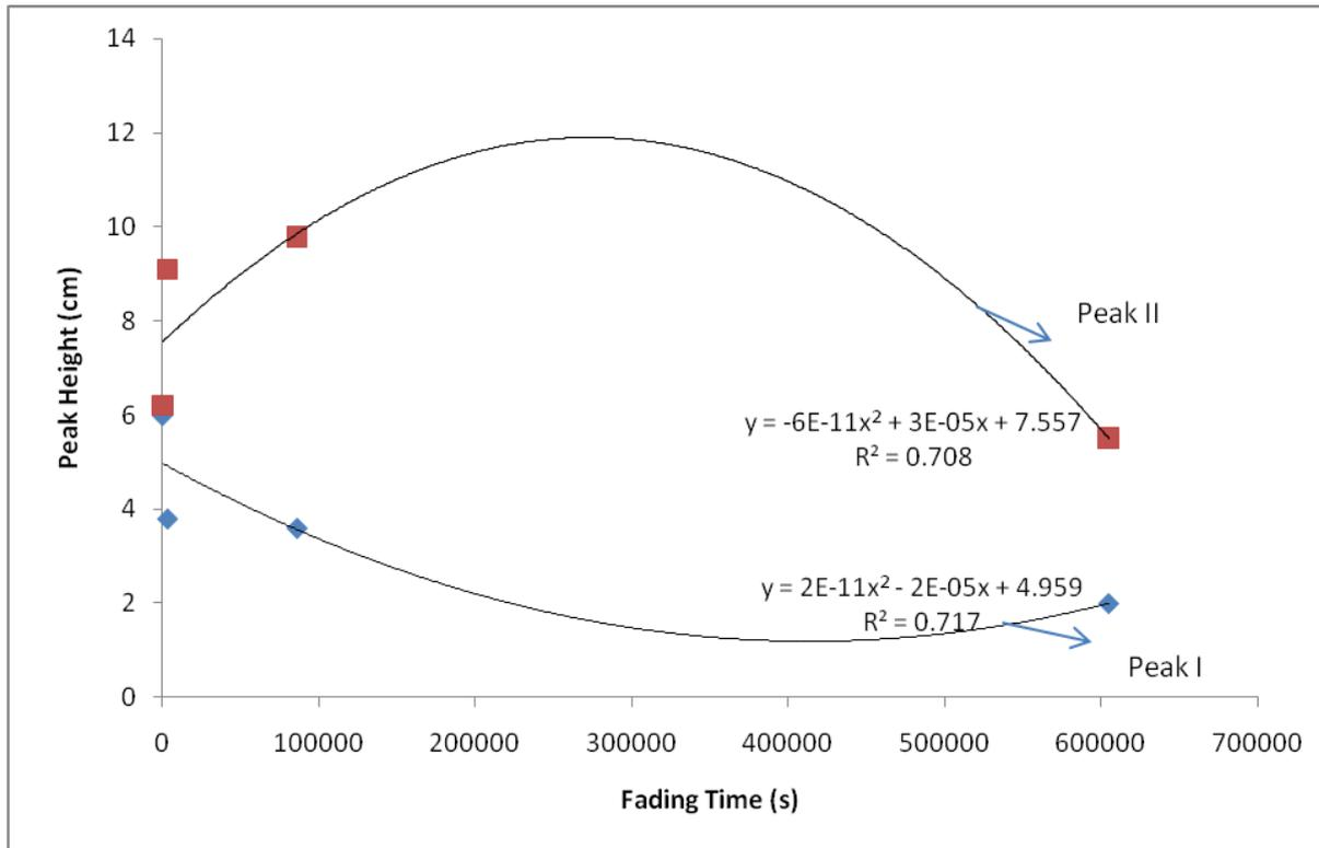
Fig. 7: Fading pattern of synthetic fused quartz with  $^{90}\text{Sr}/^{90}\text{Y}$  irradiation source
