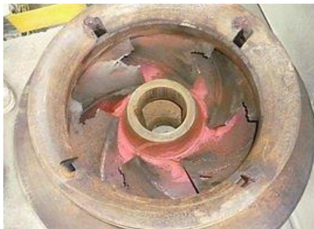
Figure 2. The cavitation of centrifugal pump impeller.
