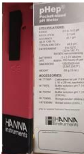
Figure - 1: showing pHep pocket sized pH meter.
