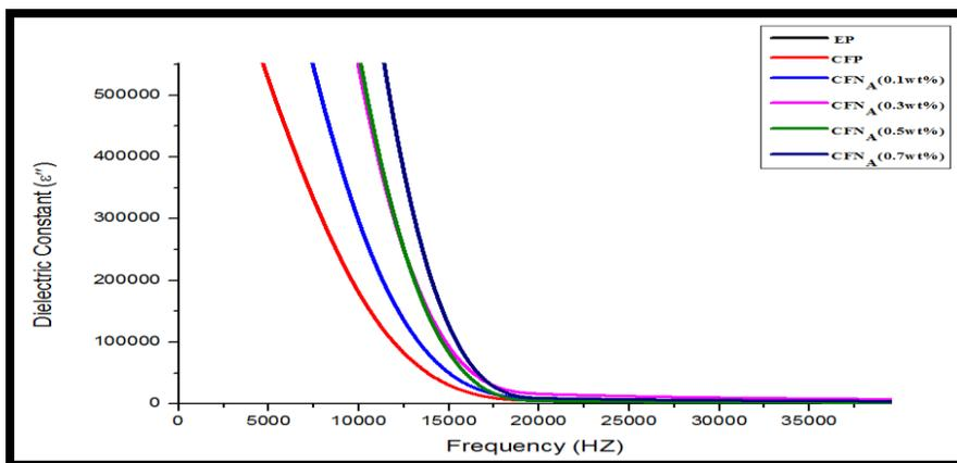
Figure 3: Isolation loss factor as a function of frequency of carbon fiber epoxy composites and alumina nanoparticles with different weight ratios.
