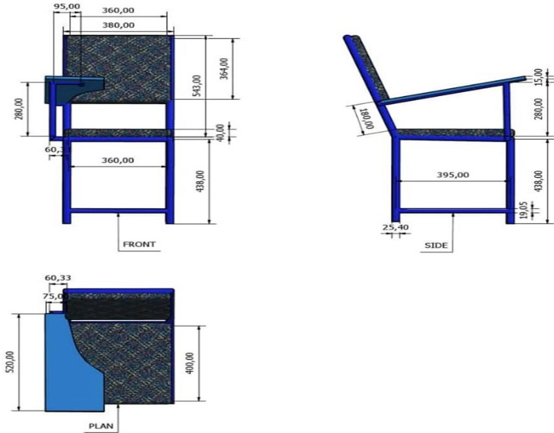
Figure 7: Orthographic projection of the model seat design
