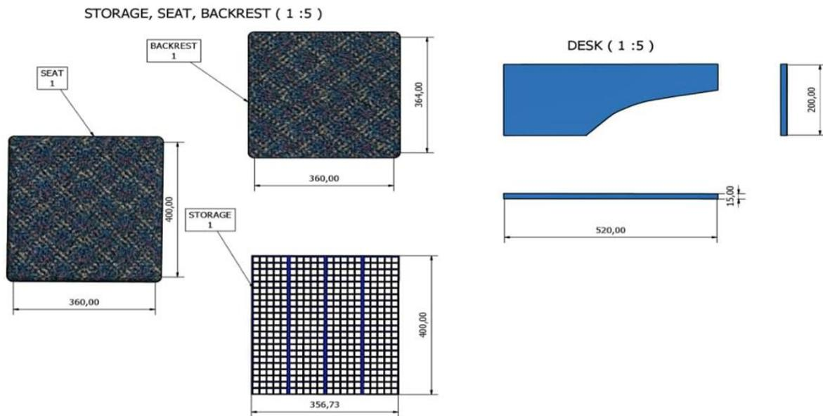
Figure 8: Exploded view of the component par
