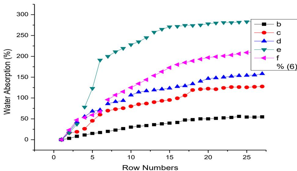
Figure 2: Water absorption of (a) untreated kapok, (b) HCl-treated, (c) NaOH-treated, (d)NaClO-treated, (e) NaClO-NaOH-NaClO-treated, and (f) NaClO<sub>2</sub>-NaOH-NaClO<sub>2</sub>-treated
