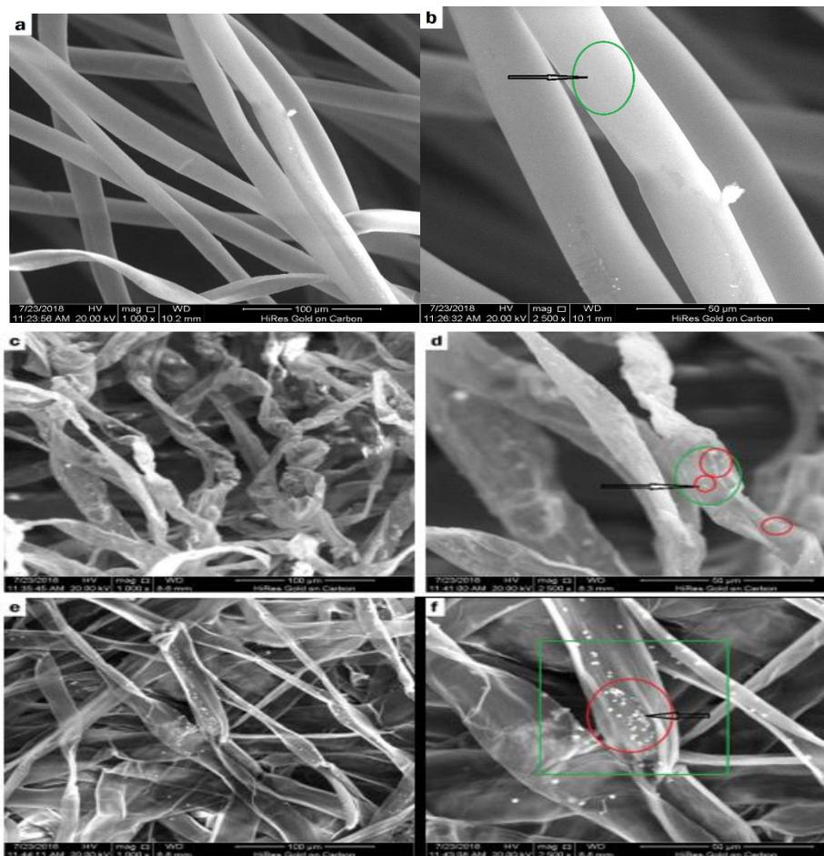
Figure 3: SEM Micrograph of (a and b) untreated kapok, (c and d) NaClO-NaOH-NaClO treated, and (e and f) NaClO<sub>2</sub>-NaOH-NaClO<sub>2</sub>-treated kapok
