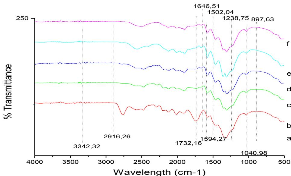
Figure 1: FTIR Spectra of (a) untreated kapok, (b) HCl-treated kapok, (c) NaOH-treated kapok, (d) NaClO-treated kapok, (e) NaClO-NaOH-NaClO-treated kapok, and (f) NaClO<sub>2</sub>-NaOH NaClO<sub>2</sub>-treated kapok
