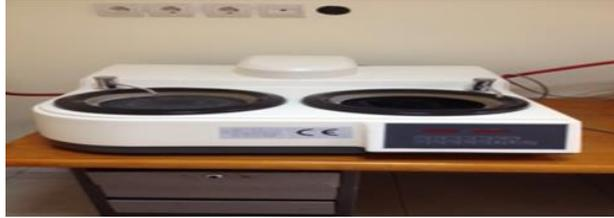
Figure 3: Sample grinding and polishing machine
