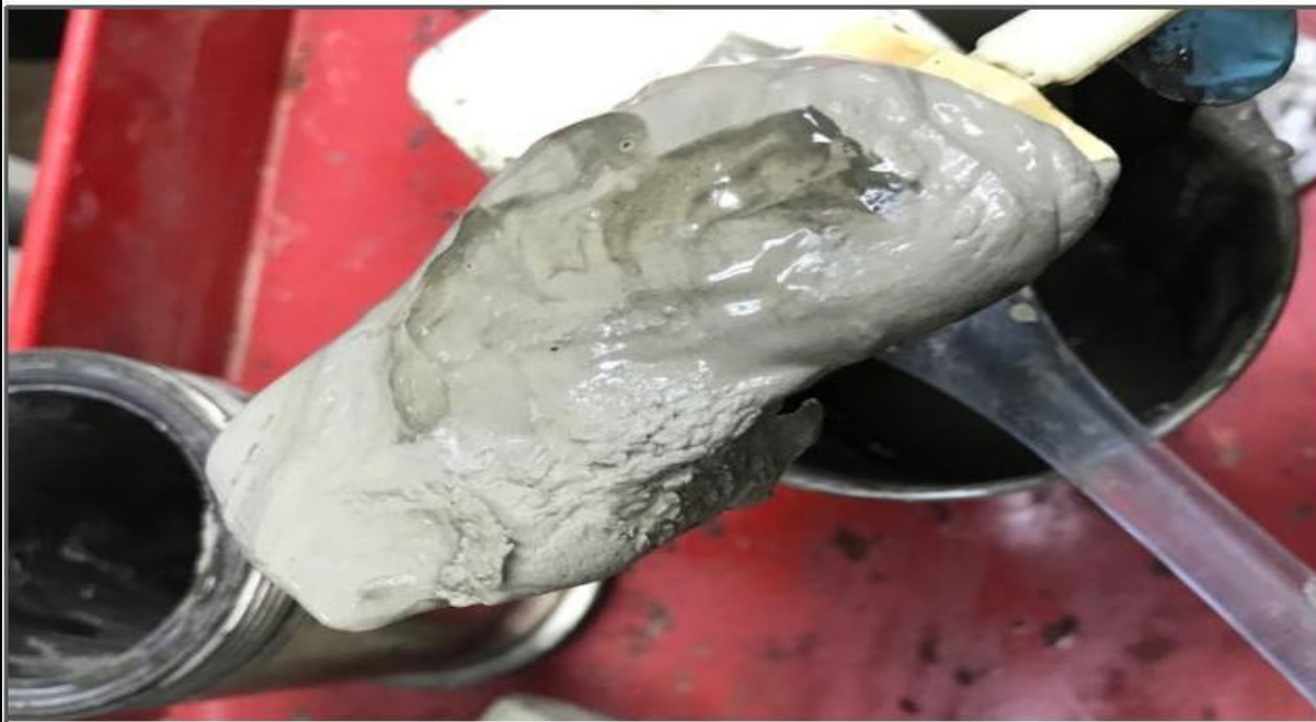
Fig. 5. Barite sagging due to low LSRV
