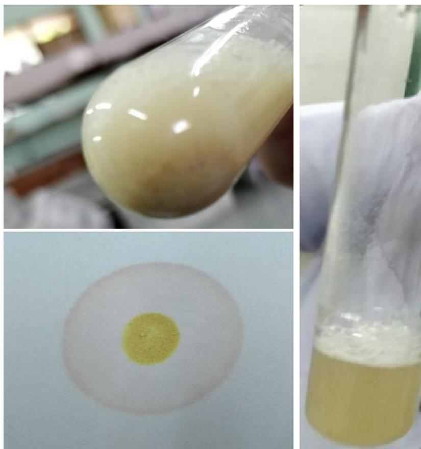
**Figure 3:** Alcohol production by Iodoform test and Qualitative test for acetic acid (presence of effervescence)
