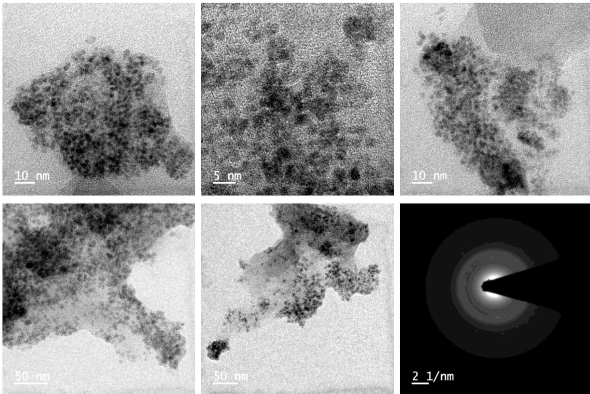
Fig. 5 HR-SEM spectra of Palladium nanoparticles
