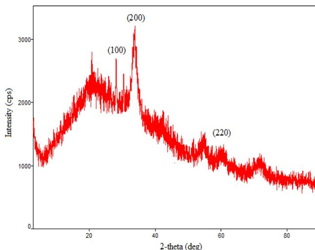
Fig. 4: XRD spectra of green synthesized Gold nanoparticles
