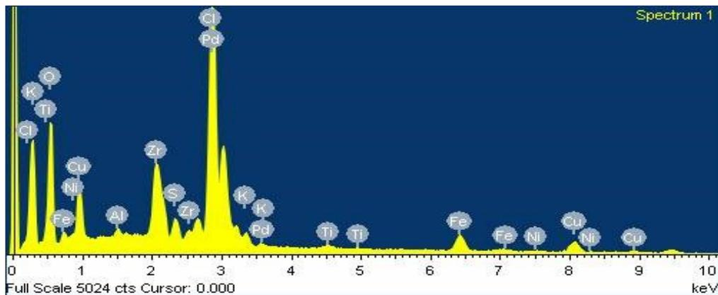
Fig. 6 EDS spectra of green synthesis of Palladium nanoparticles
