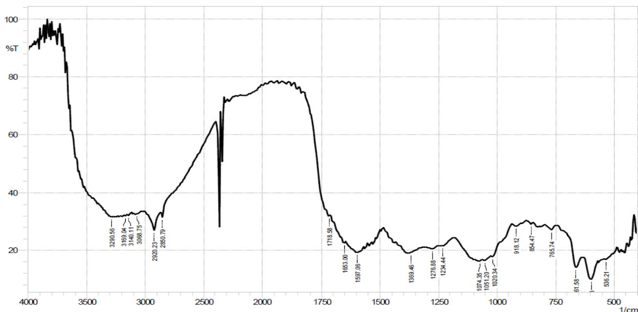
Fig3. FTIR spectrum of Palladium nanoparticles
