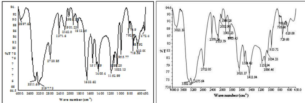
Fig. 2. FT-IR spectra for 1mole% Glycine doped ZTS
