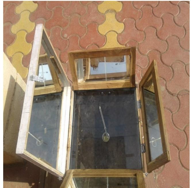
Figure 2: Typical and Experimental diagram of solar oven for observations recorded
