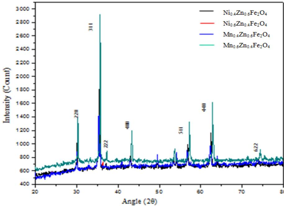
Figure 2: X-ray diffraction for composition of  $Ni_xZn_{1-x}Fe_2O_4$  and  $Mn_xZn_{1-x}Fe_2O_4$  ( $x = 0.40, 0.60$ )
