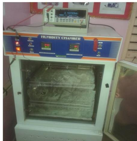
**Figure 1:** Experimental arrangement for measurement of humidity dependent characteristics of the composition under investigation.
