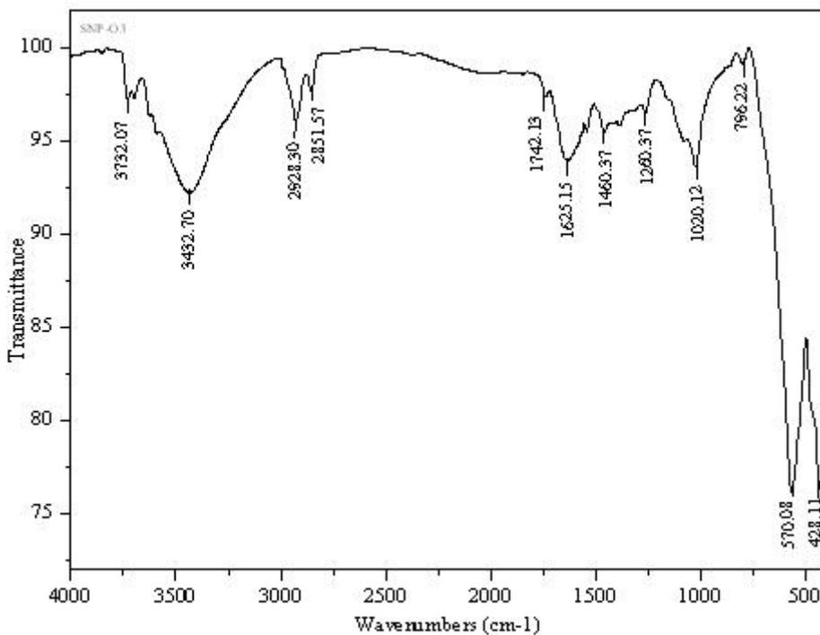
Figure 3: IR absorption spectra of the composition  $Ni_xZn_{1-x}Fe_2O_4$  ( $x=0.60$ )
