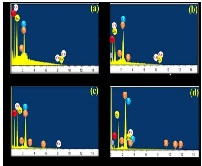
Fig. 2: EDAX images of CuBiS<sub>2</sub> NP<sub>s</sub> sensitised ZnO electrodes
