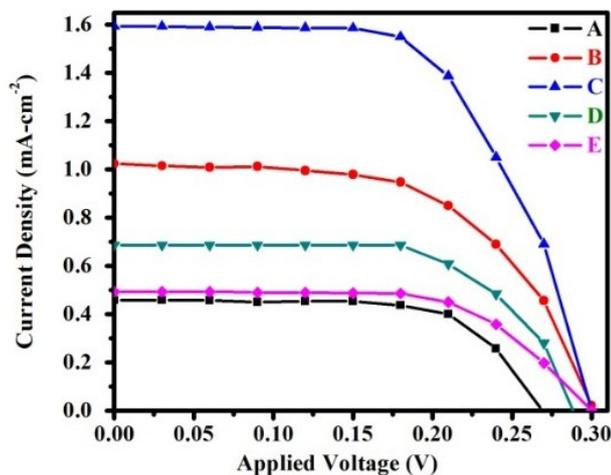
**Fig. 4:** JV analysis images of ZnO and CuBiS<sub>2</sub> NP<sub>s</sub> sensitised ZnO electrodes.
