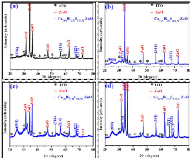
Fig. 1: XRD images of CuBiS<sub>2</sub> NP<sub>s</sub> sensitised ZnO electrodes
