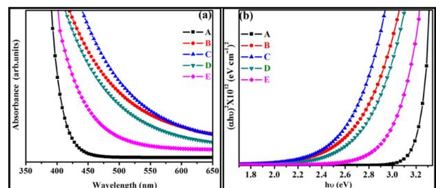
**Fig 3: (a) UV and (b) Energy band gap images of ZnO and CuBiS<sub>2</sub> NP<sub>s</sub> sensitised ZnO electrodes**
