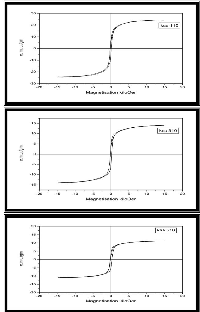
**Fig.1** Hysteresis loop of mixed ferrites  $CuFe_{2-2y}Al_{2y}O_4$  system for  $y = .05, 0.15$  and  $0.25$
