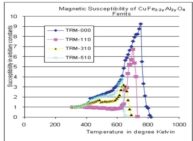
**Fig.2** Magnetic Susceptibility of mixed ferrites  $Cu Fe Al O$  system
