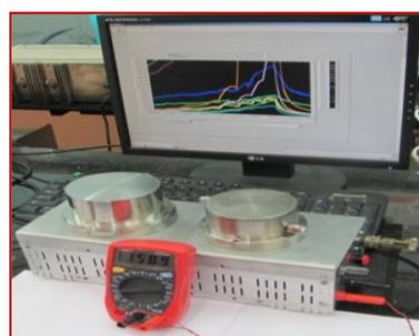
**Figure 1.** The indigenously developed table top static gas sensing unit.
