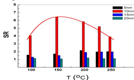
**Figure 2.** Sensor response as a function of operating temperature and Ag thicknesses.
