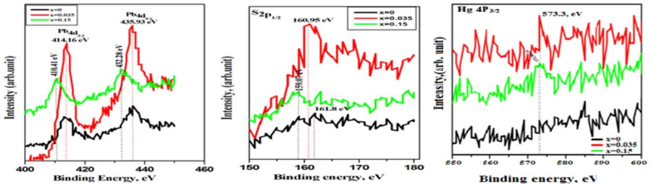
Fig.3 High-resolution XPS spectra for: (a) Pb 4d<sub>3/2</sub>, (b) S 2p<sub>1/2</sub> and (c) Hg 4p<sub>3/2</sub> regions for HgPbS thin films.
