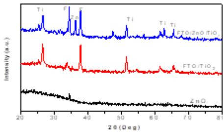
Fig.1. X-ray diffraction patterns of ZnO, TiO<sub>2</sub> and ZnO: TiO<sub>2</sub> thin films
