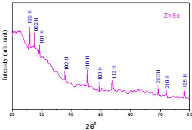
Figure 3. X-ray diffractogram of ZnSe Thin Film
