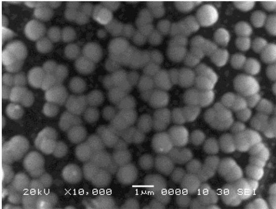
Figure 2 SEM Micrographs of ZnSe Thin Films
