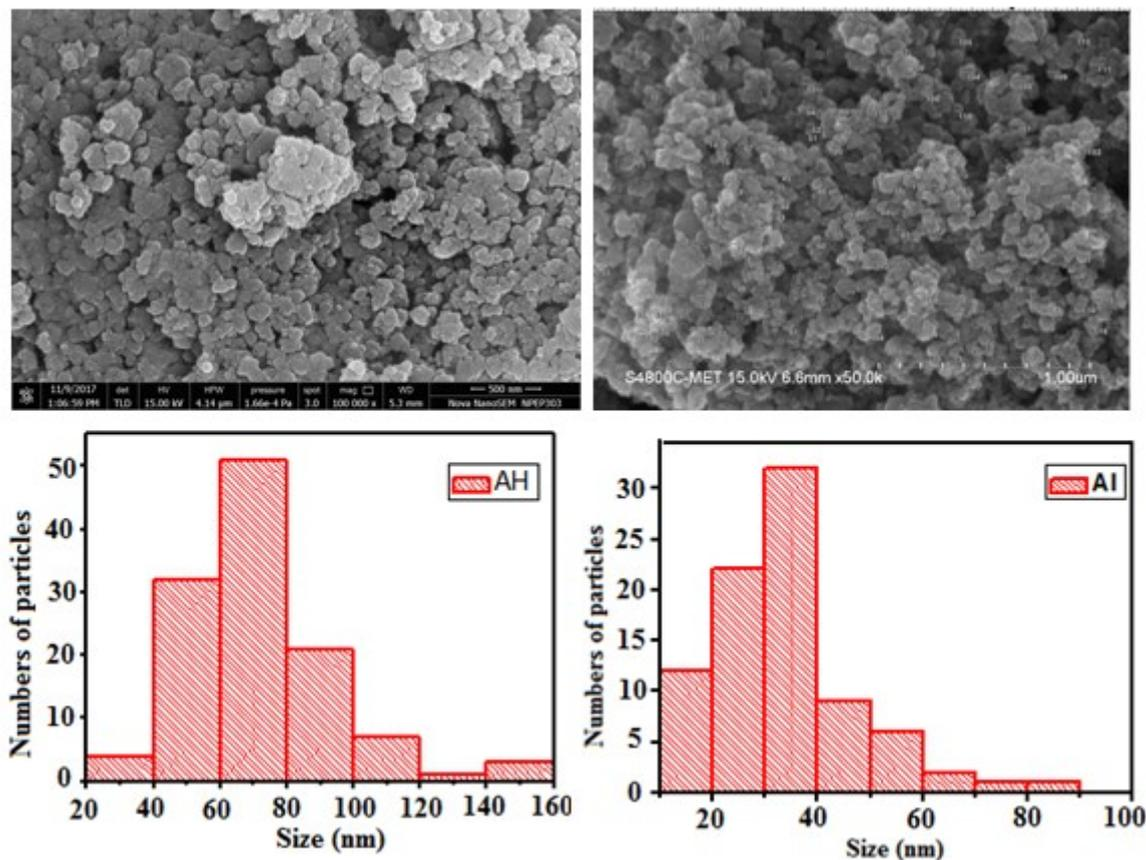
Fig. 2. The microphotographs and corresponding particle size distribution for AH450 (left) and AI450 (right) TiO<sub>2</sub> powders
