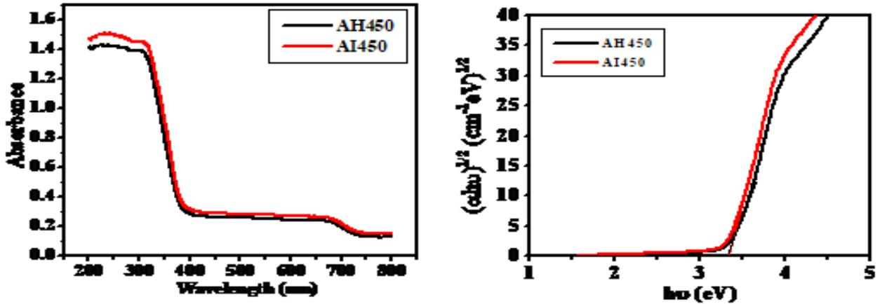
Fig 3. UV-Visible spectra and corresponding Tauc plots for AH450 and AI450 TiO<sub>2</sub> powders
