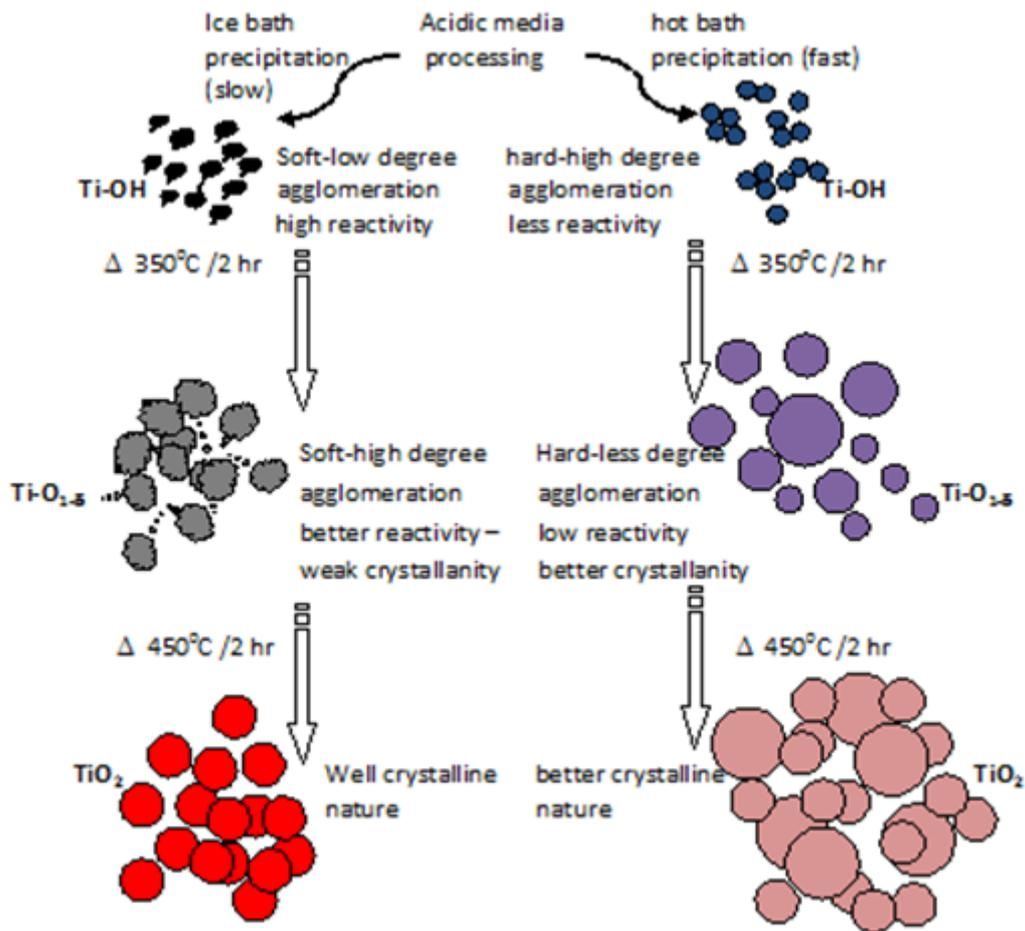
Fig. 4. The mechanism for processing of TiO<sub>2</sub> powder with anatase symmetry by using the acidic route
