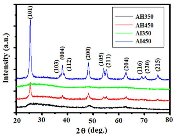
**Fig. 1.** The X-ray diffraction (XRD) patterns of pure TiO<sub>2</sub> prepared under different processing conditions
