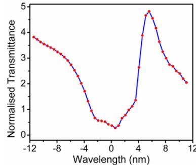
Fig.3. Closed aperture Z-scan transmittance curve of LC-ZTS
