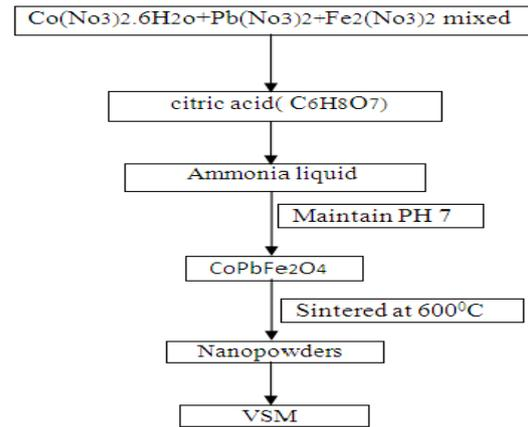
**Figure 1.** Sol-gel method for the preparation of ferrites
